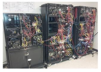
The SEPS Lab consists of three workstations. The fully reconfigurable six-bus, three phase power system hardware operates with ratings of 208 V (at 60 Hz) and 0.2 kW.
